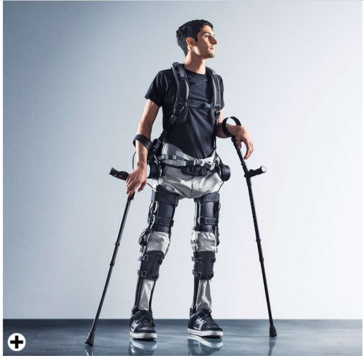
A battery pack worn as a backpack powers the exoskeleton for up to eight hours.
